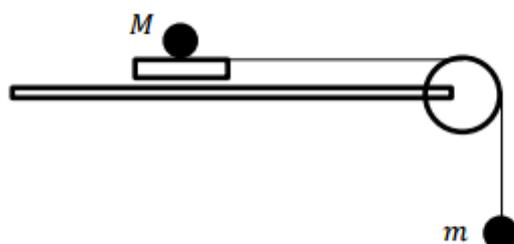
Masses are added to  $m$  until the pull on the  $M$  causes the block to slide along the table. This is repeated for different values and the results are recorded. Data of  $F$  against  $R$  are plotted for further investigation.
