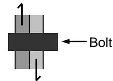
To calculate the total combined shear force on the bolts you need to summate the horizontal then vertical components of the forces independently and combine.
