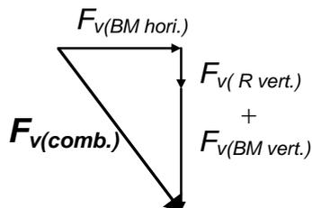
$$F_{v(comb.)} = \sqrt{(F_{v(BM \text{ hori.})})^2 + (F_{v(R \text{ hori.})})^2}$$
