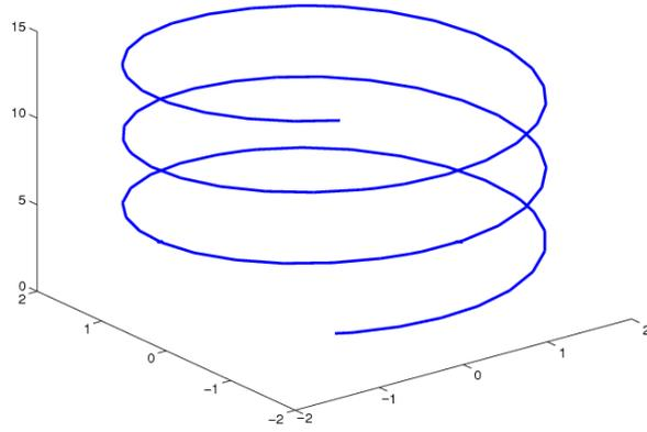
The speed of the torch relative to the part (surface speed) is always set at 381 mm/s. Now we need to calculate the traverse speed of the torch to keep on the correct flight diameter (the speed of the torch travelling along the part, which will be less than the surface speed).
