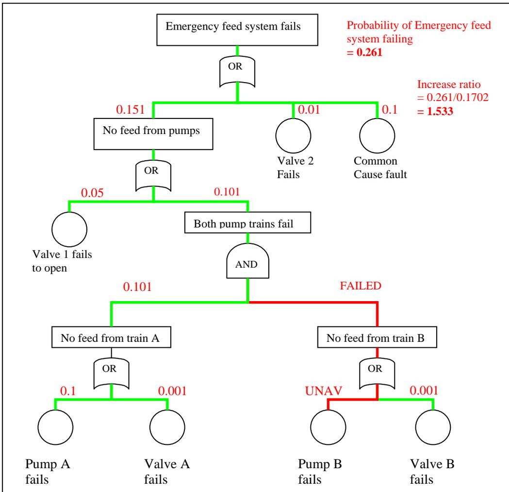
Making pump B unavailable does not fail the whole system because pump A is still functioning normally. However, the probability of the system failing has increased by a factor of 1.533 as only one pump is now available to feed the system. Therefore the operators would wish to carry out the maintenance of pump B as quickly as possible in order to keep the probability of the system failing ALARP.
