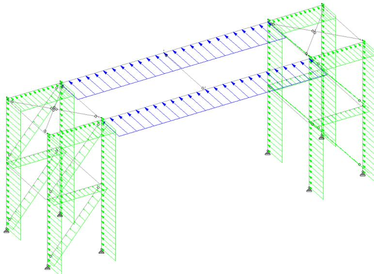
Fig 3. Wind Loadings on Support Structure model from STAADPro V8i
