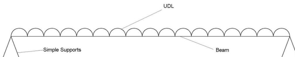
Fig 2. Simply Supported Beam with a Uniformly Distributed Load
